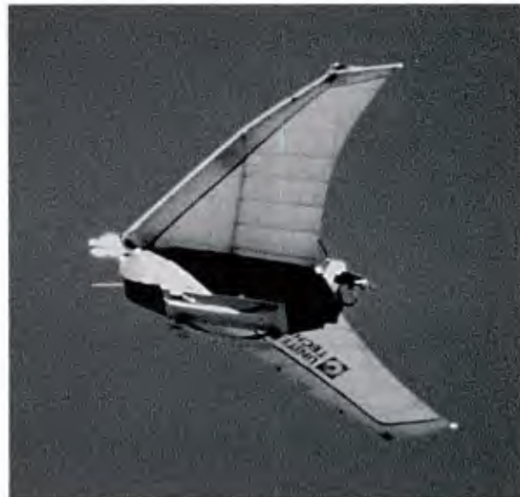
Air Delivery Systems: High-Glide, Semirigid Wing Air Delivery System, a high-altitude autonomously guided, offset cargo airdrop system that will minimize aircraft vulnerability to low-altitude threats and enhance the rapid deployment and precision delivery of sensors and munitions.
