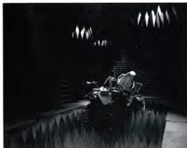
Figure VI-18. Multispectral Environmental Generator and Chamber
