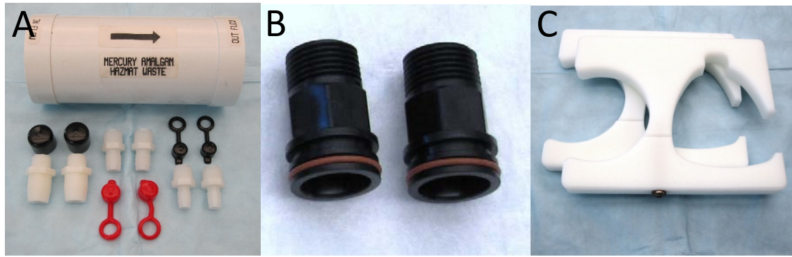
Figure 1. The DD2011P chairside amalgam separator with installation parts: (A) The DD2011P is packaged with three sets of hose barbs to accommodate different tubing sizes and vinyl caps are furnished to close off the connections when the separator is removed for disposal. (B) Quick-disconnect fittings developed by NAMRU-SA and fielded to Navy dental facilities for testing and improved convenience of installation. (C) Mounting brackets which anchor the separator to the back of A-dec 500-series chairs.
