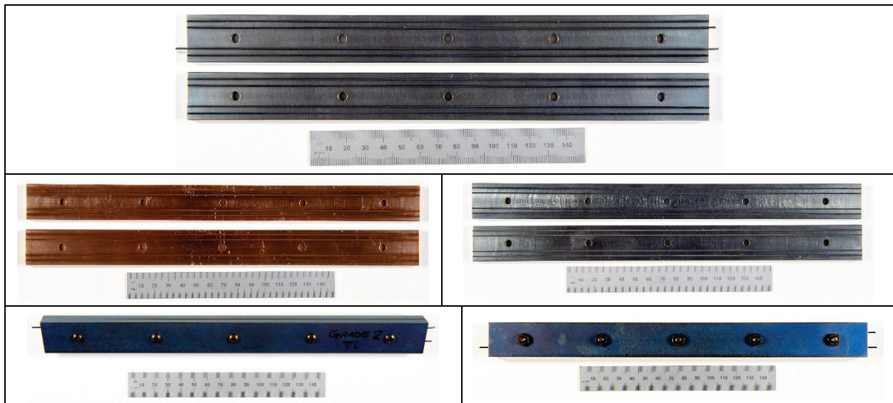
Figure 7: Stress-relief fixtures for straightening the wire samples. (Top and middle) inside view of the Ti, Cu, and Fe fixtures showing four “wire-tracks”; and (bottom) exterior view of the Ti fixture clamped and bolted.
