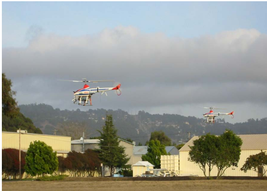
Figure 2. Pilot-Directed Computer Assisted Helicopter Formation Flying.
