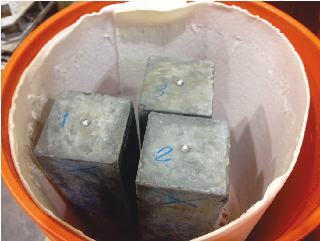
Figure 3. Prisms in a sealed container at 38 °C and > 95% RH in accordance with ASTM C1293.
