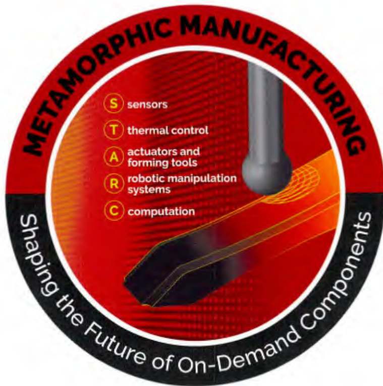
Figure 1. Synopsized illustration of metamorphic manufacturing (MM), including the five fundamental elements represented by the acronym STARC (Sensors; Thermal control; Actuators and forming tools; Robotic manipulation systems; Computation).
