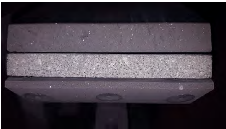
Figure 28. Model with SiC-coated C-C sample after shot x2s3576.
