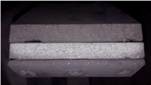
(b) SiC-coated sample after shot x2s3833
