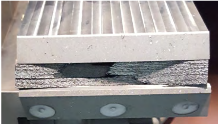
Figure 19. Model with C-C sample after shot x2s3564.
