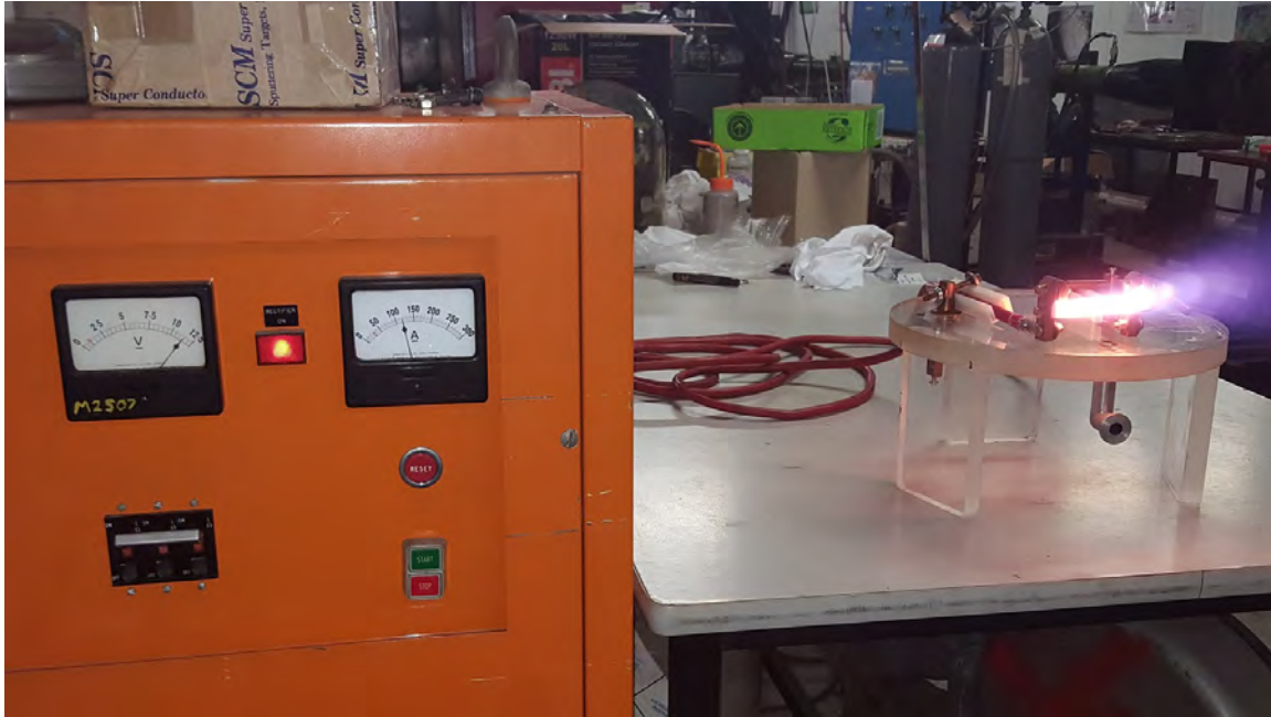
Figure 14. Power supply used for bench testing. Sample being heated was C-C.
