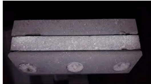
(c) Reused SiC-coated sample after shot x2s3834
