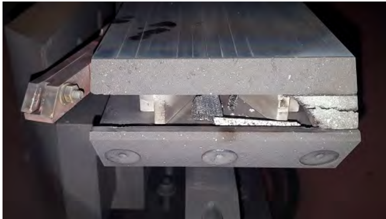
Figure 24. Model with SiC-coated C-C sample after shot x2s3572.
