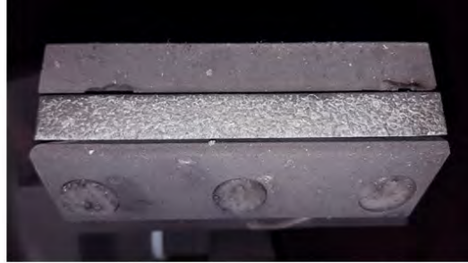
(a) Unused SiC-coated sample before shot x2s3833
