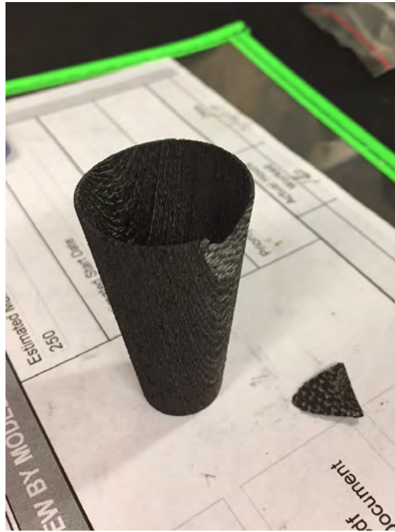
Figure 136. Attempt at machining a 3D cone out of C-C.
