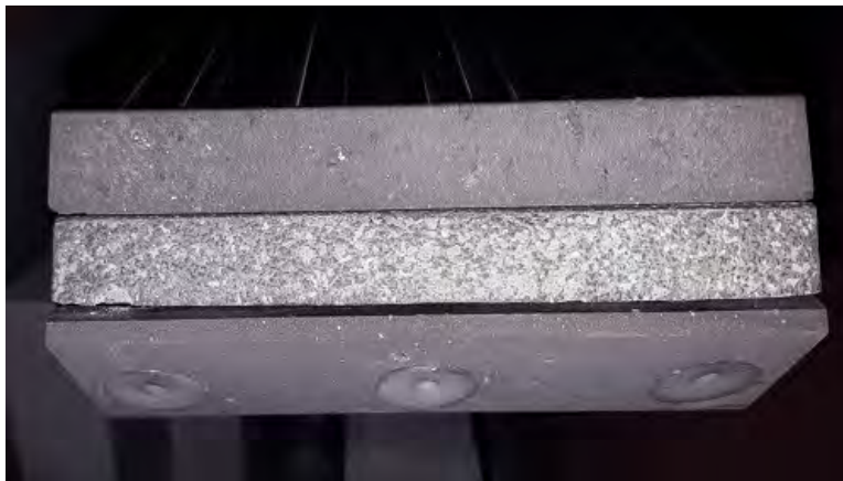
Figure 22. Model with SiC-coated C-C sample before shot x2s3572.
