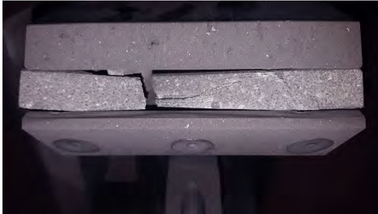
Figure 26. Model with SiC-coated C-C sample after shot x2s3574.
