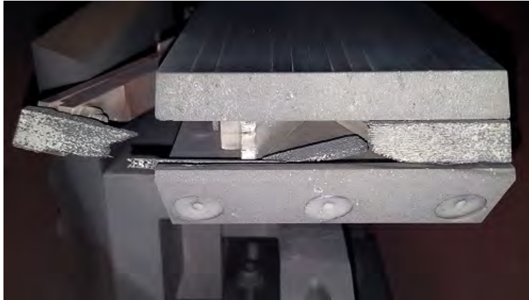
Figure 23. Model with SiC-coated C-C sample after shot x2s3571.
