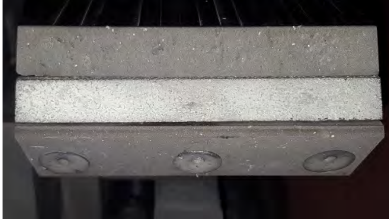
Figure 29. Model with SiC-coated C-C sample after shot x2s3577.
