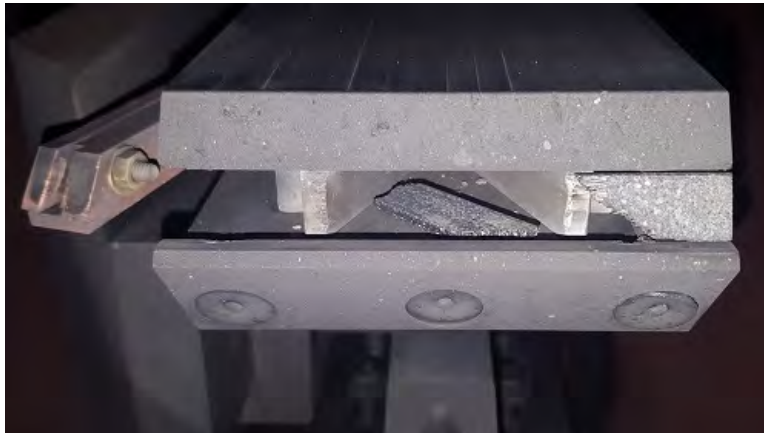
Figure 27. Model with SiC-coated C-C sample after shot x2s3575.
