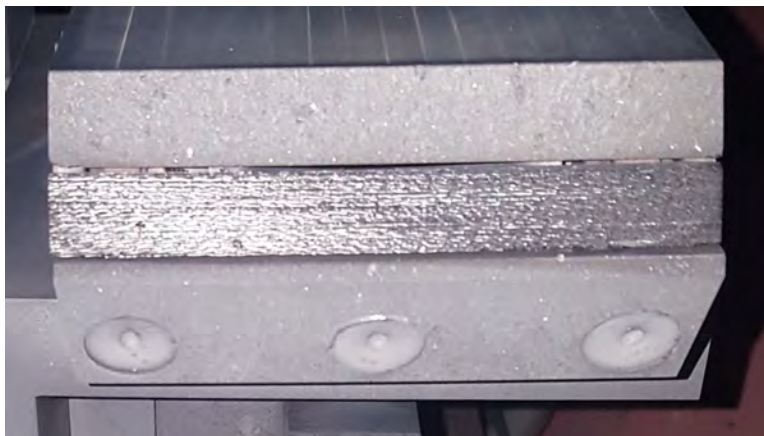
Figure 21. Model with C-C sample after shot x2s3570.
