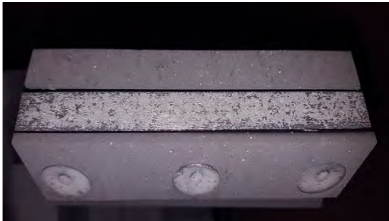
Figure 30. Model with SiC-coated C-C sample after shot x2s3578.
