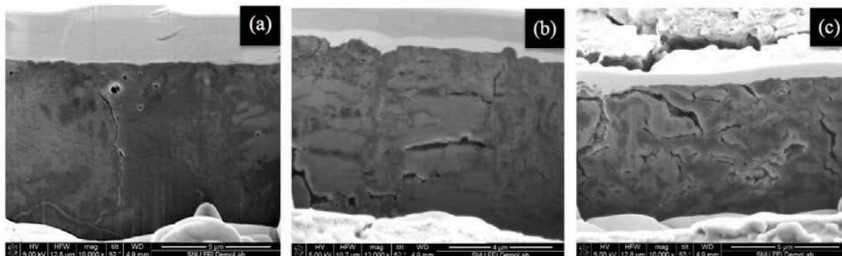
Figure 16. FIB Cross Sectional Views of Si-C:SSE Composite Electrodes After 100 Charge-Discharge Cycles, (a) 6:4 nSi-C:SSE Composite Electrode, (b) 7:3 nSi-C:SSE Composite Electrode, and (c) 7:3 Si-C:SSE Composite Electrode Containing 1-3 \mu\text{m} Silicon Particles
