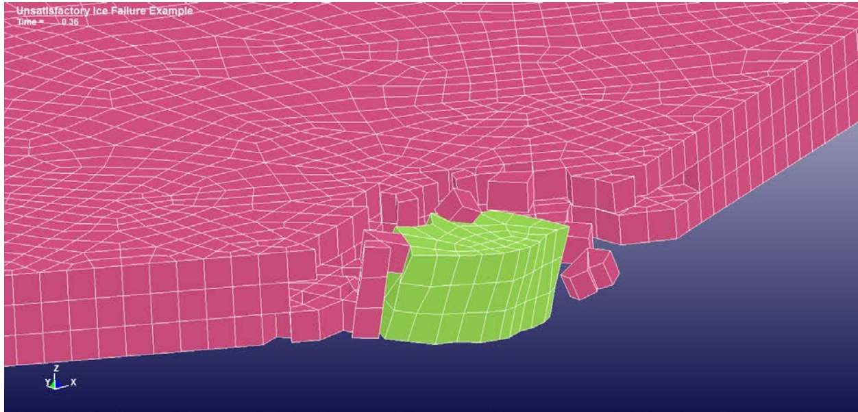
Figure 11. Example of Unsatisfactory LS-DYNA-Computed Ice Slab Failure Using a Crushing Calibration Study Ice FEM
