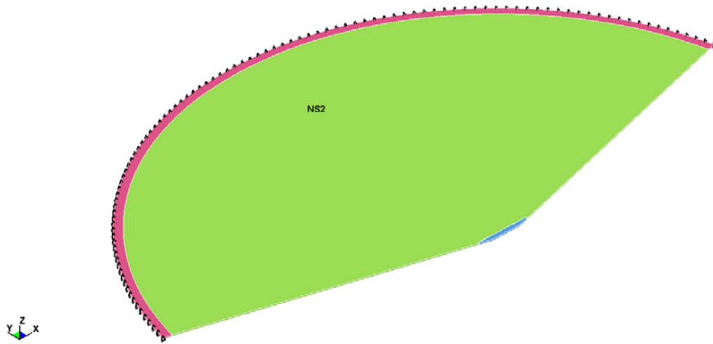
Figure 5. Nodal Constraints Applied to Ice Slab FEMs
