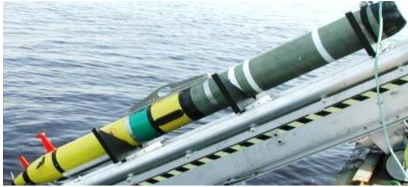
Figure 1 – Prototype LSG sensor mounted on a REMUS600 being deployed in the field.
