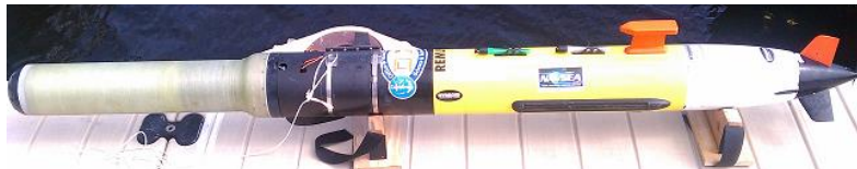
Figure 2 – Prototype single axis gradiometer mounted on a REMUS100.
