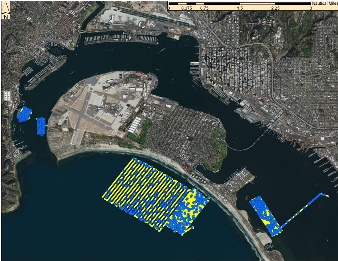
Figure 21 – Tracklines and contacts from the 2017 San Diego UXO survey.
