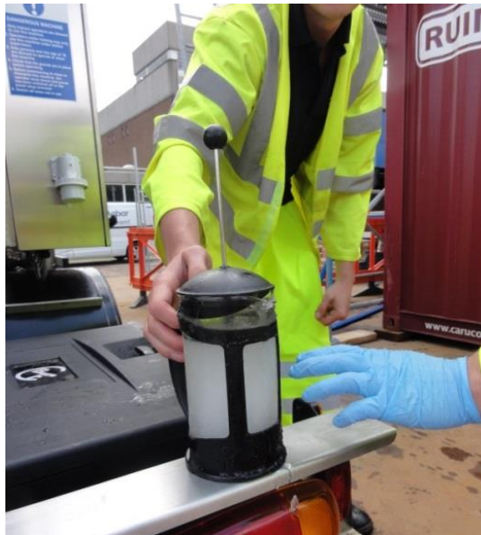
Figure 2. French Press Method of Testing the Ice Fraction
