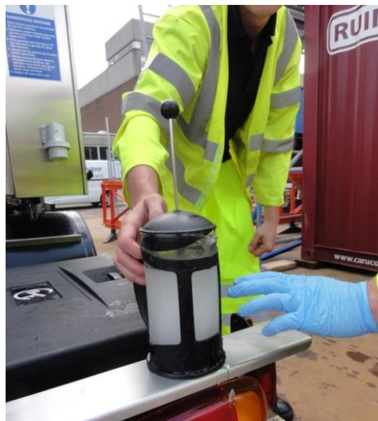
Figure E-2. French Press Method of Testing the Ice Fraction
