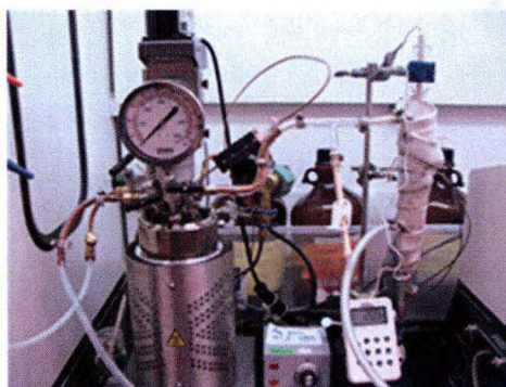
Fig 2.5.2. Laboratory setup of the dual reactor system
