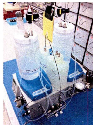
Figure 1.1.17 Schematic of liquid supply and delivery system (left) and photo of system (right)
