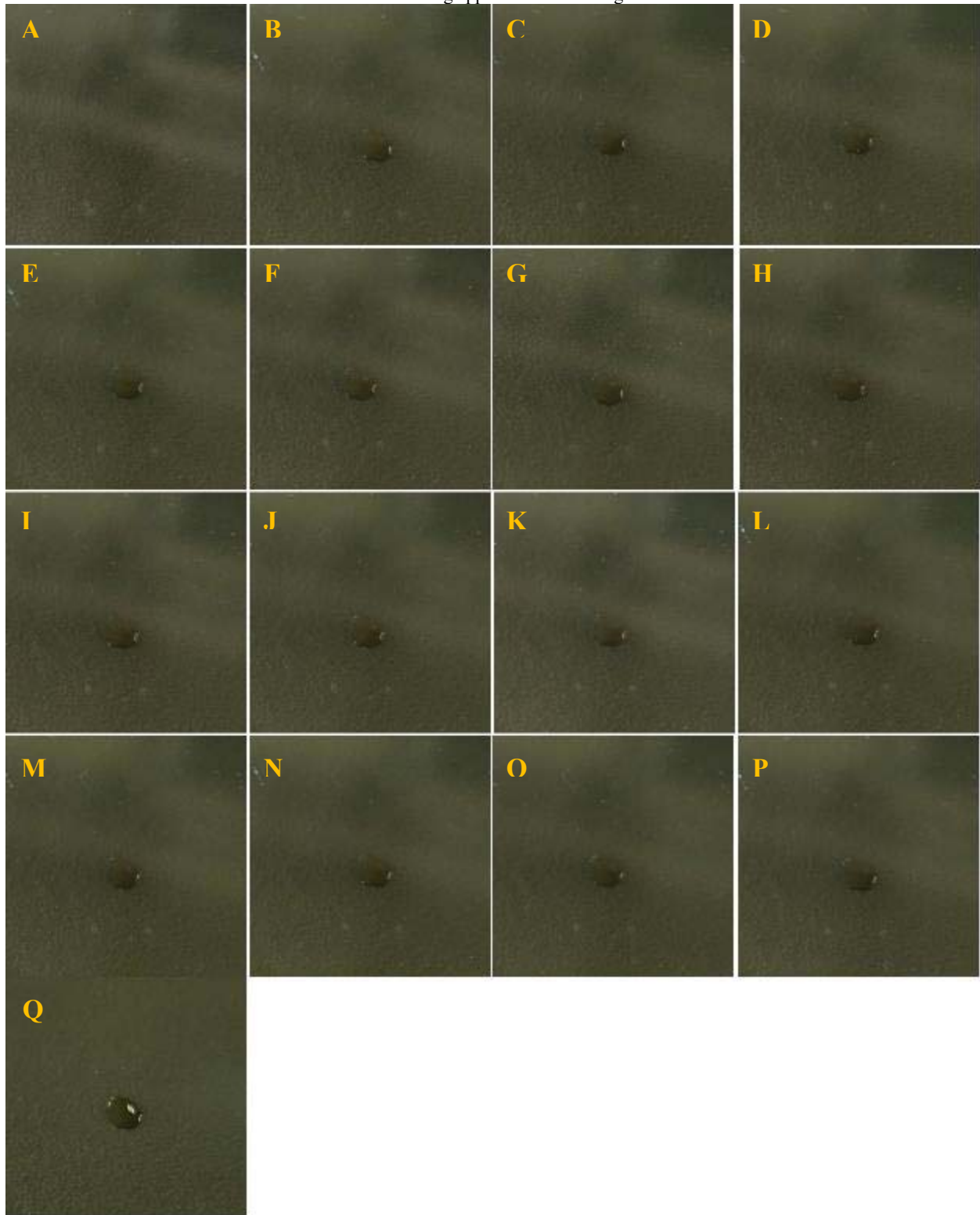
Fig. G1 — DFP on SOCAL-ARSiO, as synthesized, 270 mm/min, no lubrication. Images of a coupon before application (A) and at 0 (B), 0.5 (C), 1 (D), 1.5 (E), 2 (F), 2.5 (G), 3 (H), 3.5 (I), 4 (J), 4.5 (K), 5 (L), 10 (M), 15 (N), 20 (O), 25 (P), and 30 (Q) min following application of the target.
