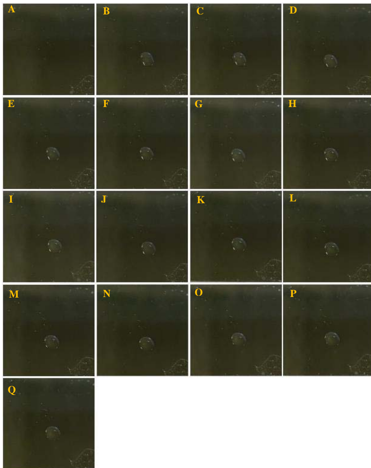
Fig. E1 — DFP on Optool. Images of a coupon before application (A) and at 0 (B), 0.5 (C), 1.0 (D), 1.5 (E), 2.0 (F), 2.5 (G), 3.0 (H), 3.5 (I), 4.0 (J), 4.5 (K), 5 (L), 10 (M), 15 (N), 20 (O), 25 (P), and 30 (Q) min following application of the target. These images were collected with a glass cover in place to limit evaporation. Reflections from the cover can be seen in some images.
