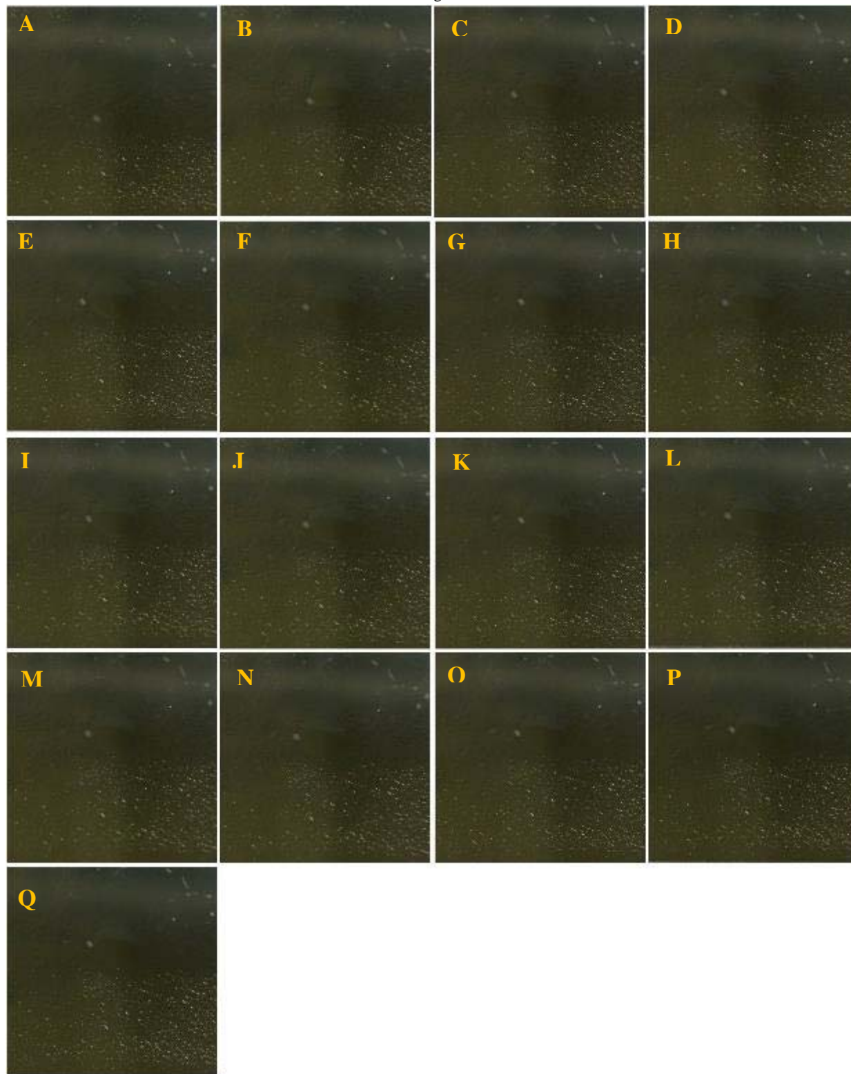
Fig. D1 — DFP on SO1455 (solvent). Images of a coupon before application (A) and at 0 (B), 0.5 (C), 1.0 (D), 1.5 (E), 2.0 (F), 2.5 (G), 3.0 (H), 3.5 (I), 4.0 (J), 4.5 (K), 5 (L), 10 (M), 15 (N), 20 (O), 25 (P), and 30 (Q) min following application of the target. These images were collected with a glass cover in place to limit evaporation. Reflections from the cover can be seen in some images.
