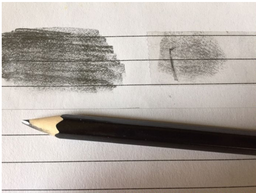
Fig. 21 “Old-school” finger printing using graphite from a pencil and a piece of clear adhesive tape
