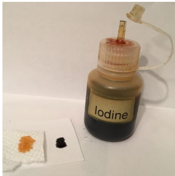
Fig. 12 Photo of a negative iodine starch response for paper towel (left, brown color) and positive response for printer paper (right, black color)
