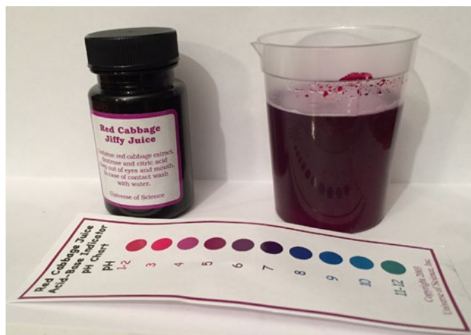
Fig. 13 Commercially available dried cabbage juice extract, reconstituted with water (right). Color/pH chart shown at bottom.
