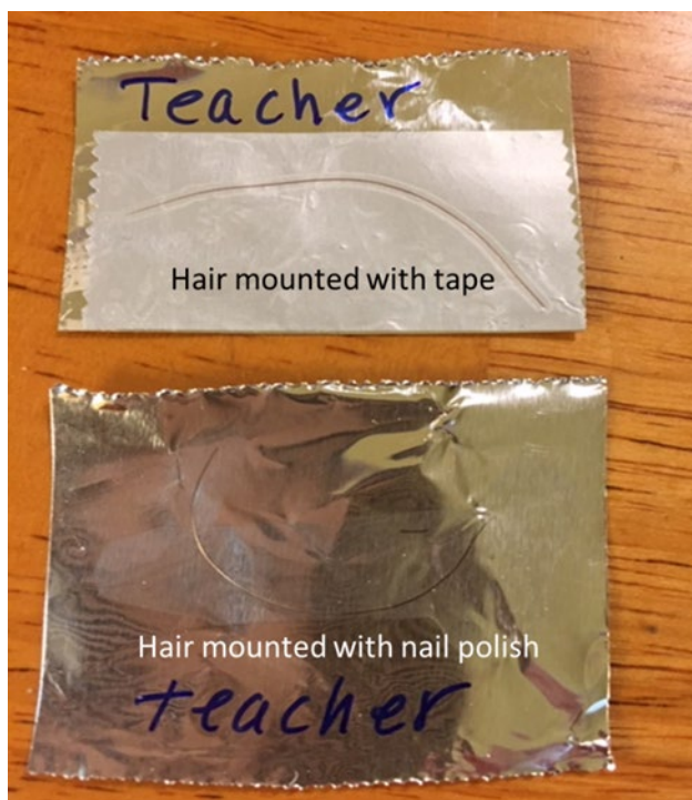
Fig. 17 Photo of hair mounted on foil with tape and clear nail polish
