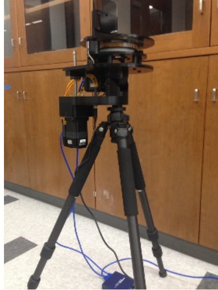
Fig. 3: AZ/EL turntable allowing mechanical steering of the radio head. The current system uses horn antennas, and thus mechanical steering is required to control the direction of transmission/reception. The turntable can be controlled using LabVIEW, which is the language used for implementing the signal processing part, and thus can be integrated into one application.
