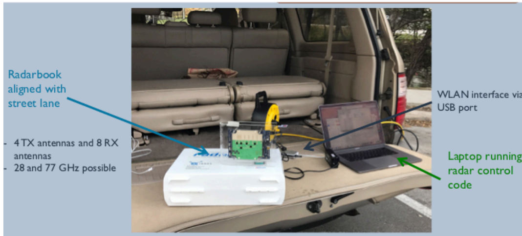
Figure 9: RadarBook setup as used for initial outdoor measurements.
