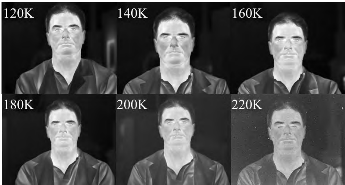
Figure 3: Infrared images taken with an AIM p-on-n MWIR MCT FPA of a person (2-point corrected, with bad pixel replacement) for detector operating temperatures between 120K and 220K. The detector's cut-off wavelength is 5.25 \mu\text{m} at 80K.
