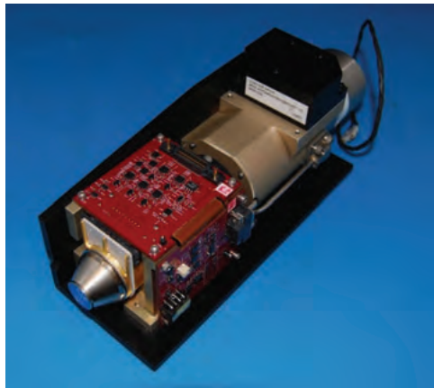
Figure 3. Photograph of the IDCA. The total mass is <1kg including the bracket and magnet shield. The total electrical power is <6W with detector chip temperature set at 110K and the heat sink (the bracket) at room temperature.
