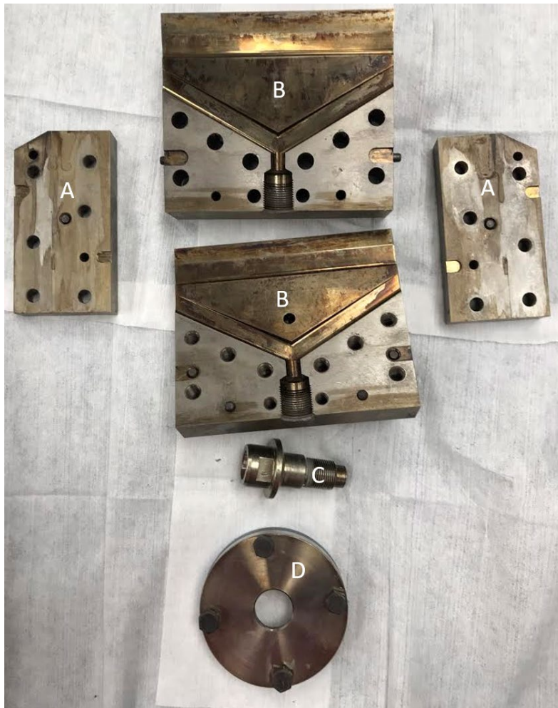
Fig. 9 A) side walls, B) top and bottom sections, C) feed port into the die, and D) rotating locking mechanism with polymer removed and surface cleaned
