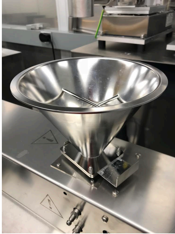
Fig. 2 Gravity feeder attached to a single-screw extruder
