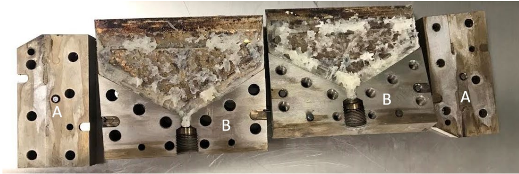
Fig. 8 Die deconstructed to its individual components, A) side walls and B) top and bottom sections, with residual polymer prior to cleaning
