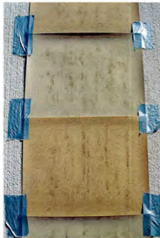
Resulting sandpaper surfaces after nine pulls: Notice black coating deposits
