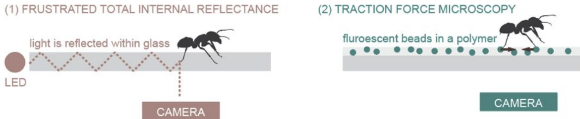
Figure 1. Two measurement techniques explored for contact mechanics observation of small-mass runners.
