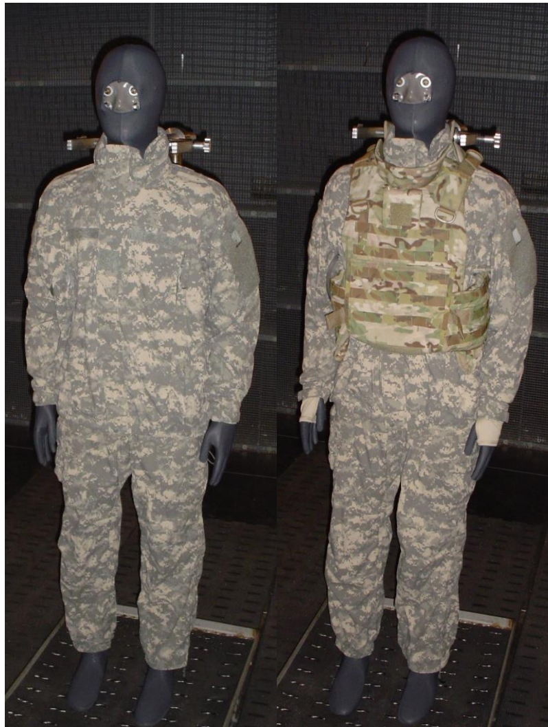
Figure 1: Images of the outer layer of the clothing worn that was used in the simulations. Left: extreme cold wet jacket and trousers. Right: extreme cold wet jacket and trousers with IOTV.
