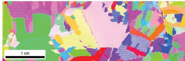
Figure 2. EBSD data collected over this sample. The colors represent the orientation of each crystal with respect to the normal direction of the surface, mapped using an inverse pole figure (IPF). This image was originally shown in [7].
