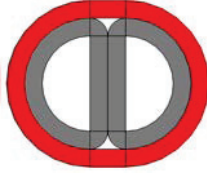
Figure 1. Image of the reflection differential coil configuration. The outside (red) coil is the excitation coil and the inside, d-shaped differential coils (grey) are the receive coils. The receive coils are counter-wound and wired in series.
