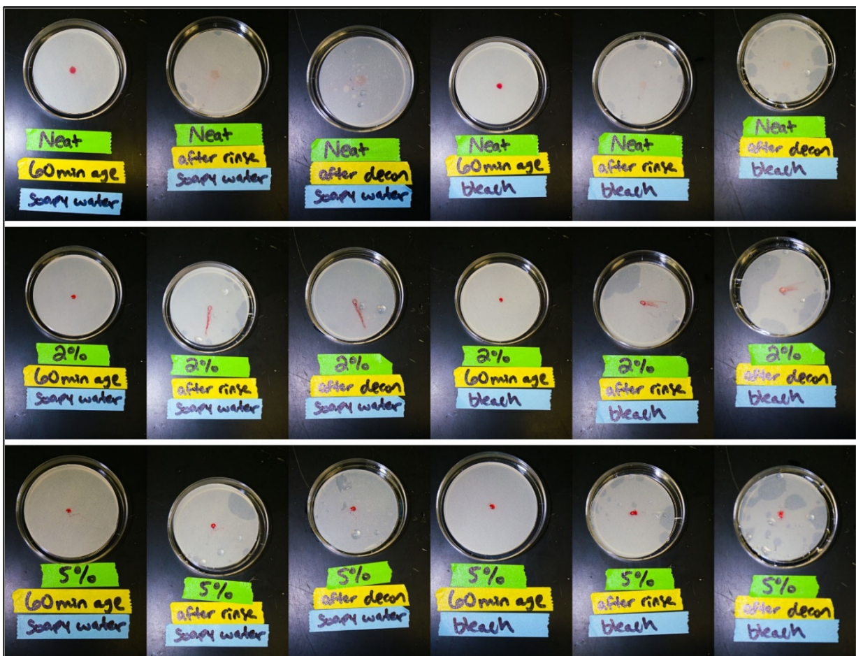
Figure 6. Images of silicone panels contaminated with 0, 2, and 5% dyed MeS thickener and treated with soapy water or bleach.
