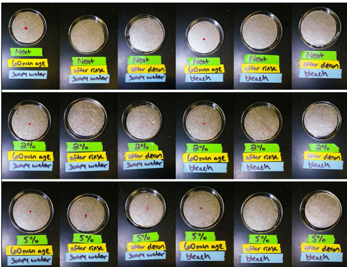
Figure 7. Images of steel panels contaminated with 0, 2, and 5% dyed MeS thickener and treated with soapy water or bleach.
