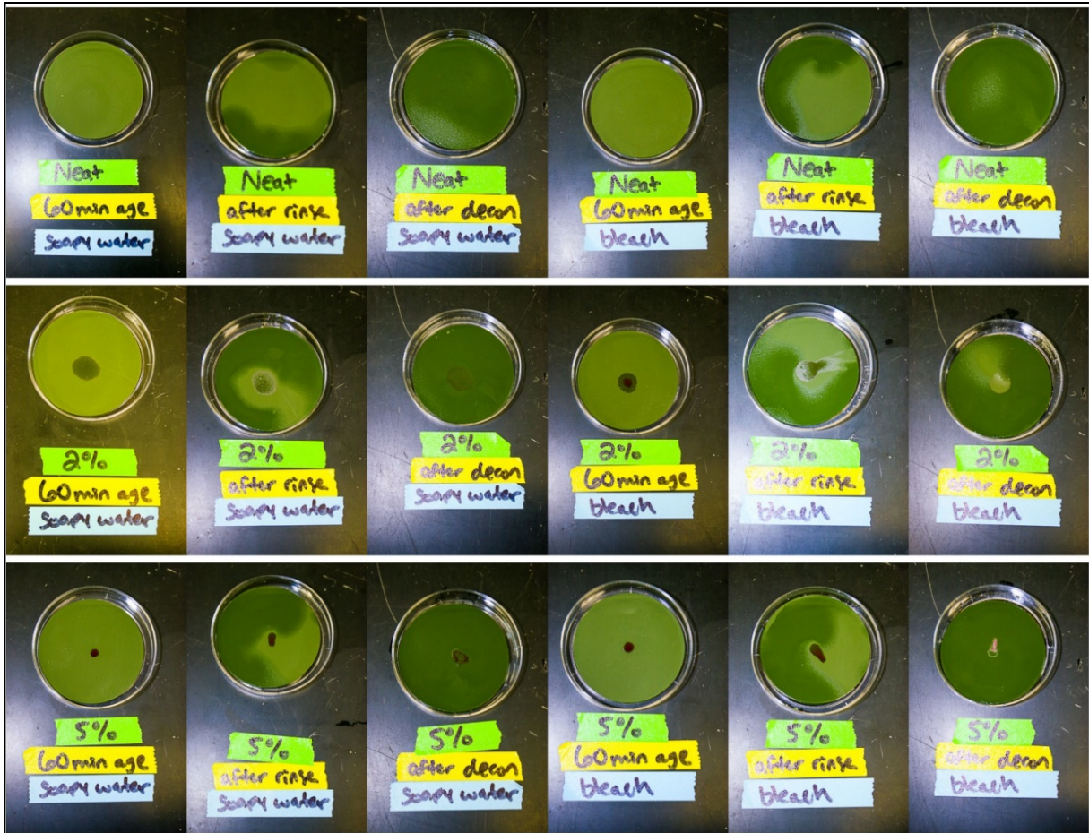
Figure 5. Images of PU-coated panels contaminated with 0, 2, and 5% dyed MeS thickener and treated with soapy water or bleach.
