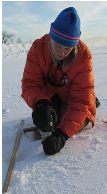
Figure 23. Snow density test on groomed snow in Michigan.
