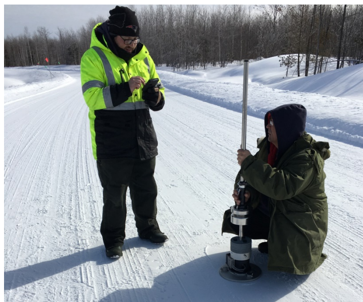
Figure 6. LWD operation in Michigan. The LWD unit and the first operator are on the right , and the second operator with the PDA is to the left .
