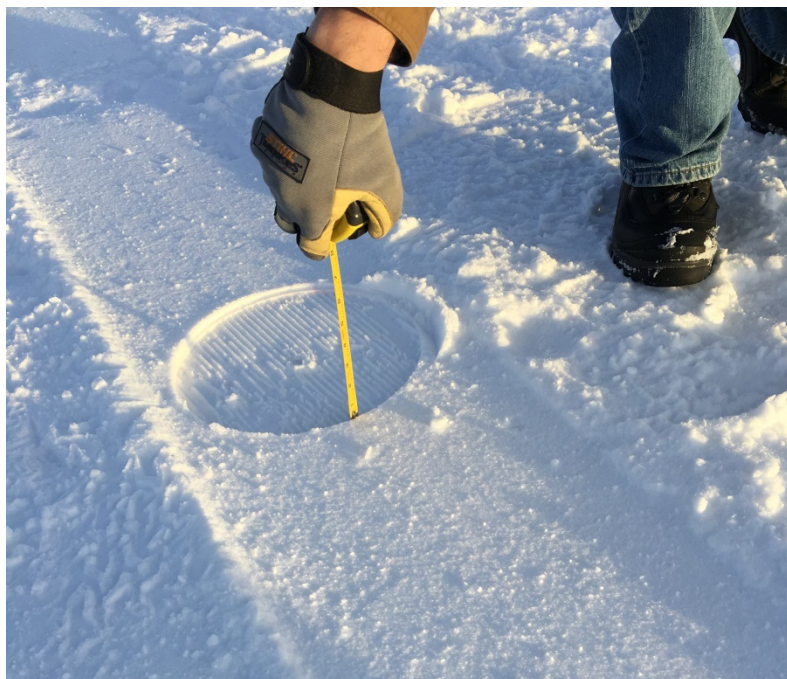
Figure 16. Impression left in the snow surface by an LWD test in Montana.
