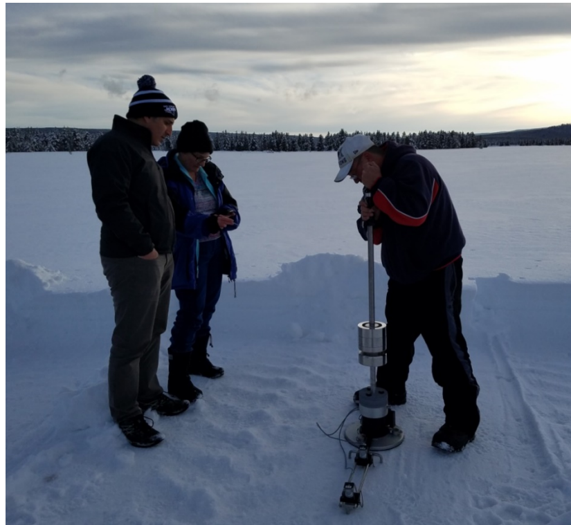
Figure 9. Initial LWD tests on groomed snow over an unpaved ground surface.
