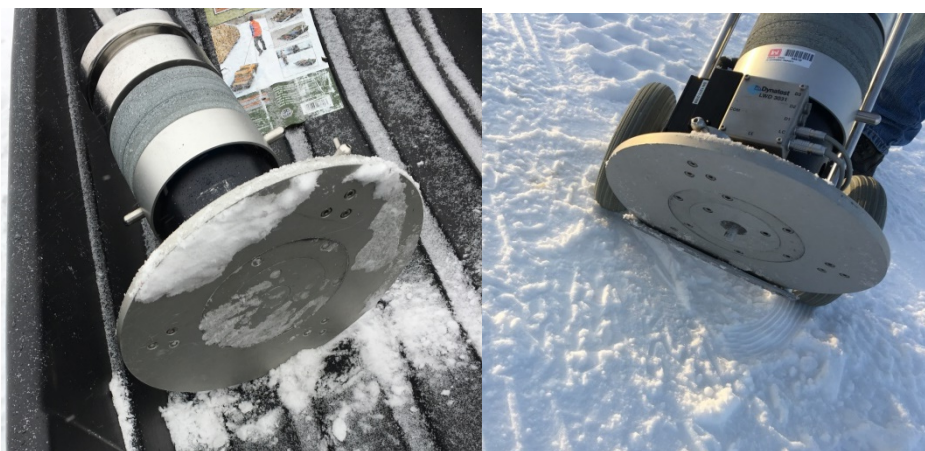
Figure 8. Dynatest LWD with the center plug in ( left ) and out ( right ) with the center plate geophone extending through the loading plate annulus.
