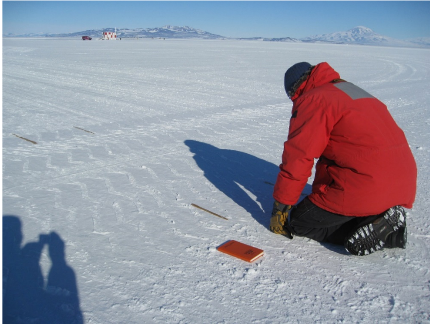
Figure 46. Two examples of pavement areas fitting the Fully Supporting performance level: ( top ) faint tire tread and ( bottom ) obvious tread and imprints.
