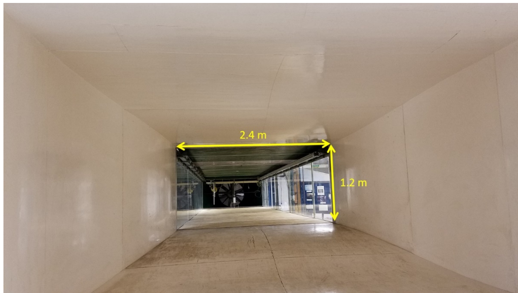
Figure 4. Inner dimensions of the contraction cone of the CRREL EWT.
