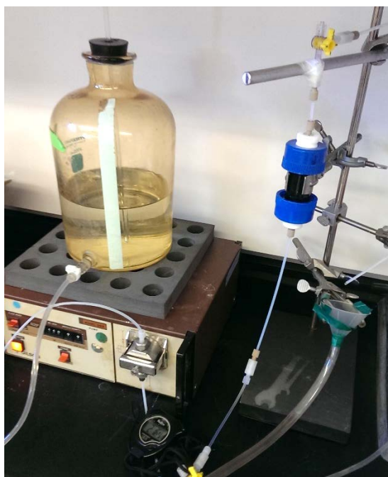
Figure 3-2. Column test setup.
