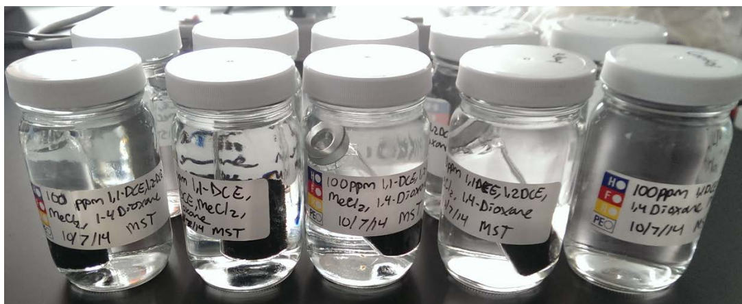
Figure 5-2. Image of the static diffusion batch test setup.
