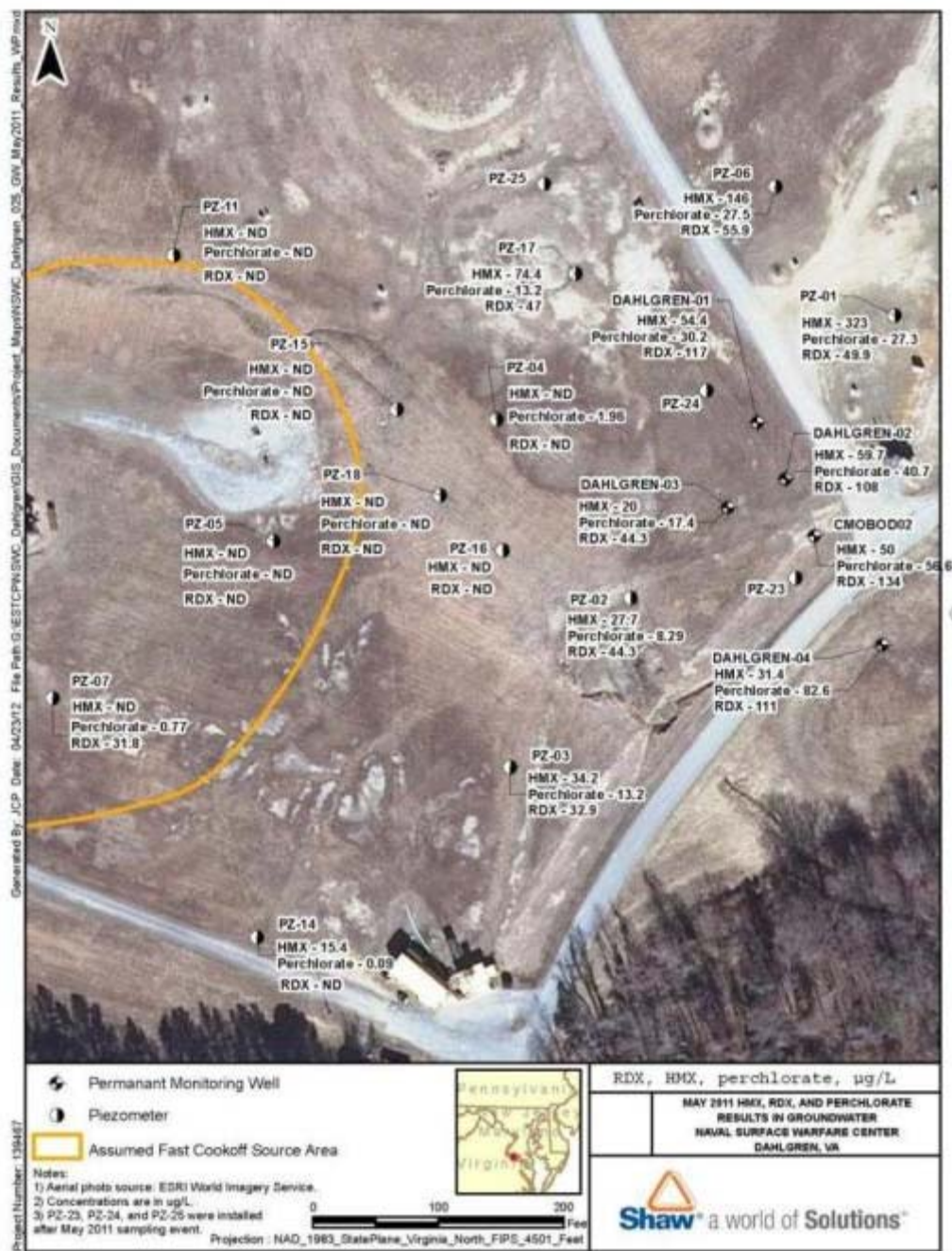
Figure 4.12. RDX, HMX and Perchlorate Data from Piezometers Installed During the May 2011 Site Investigation.
