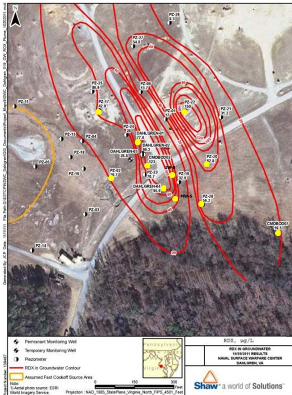
Figure 5.14. Plume Map for RDX in the Southeast Area of the Churchill Range with Locations Demarcated (yellow well markers) for the First Round of Stable Isotope Sampling.
