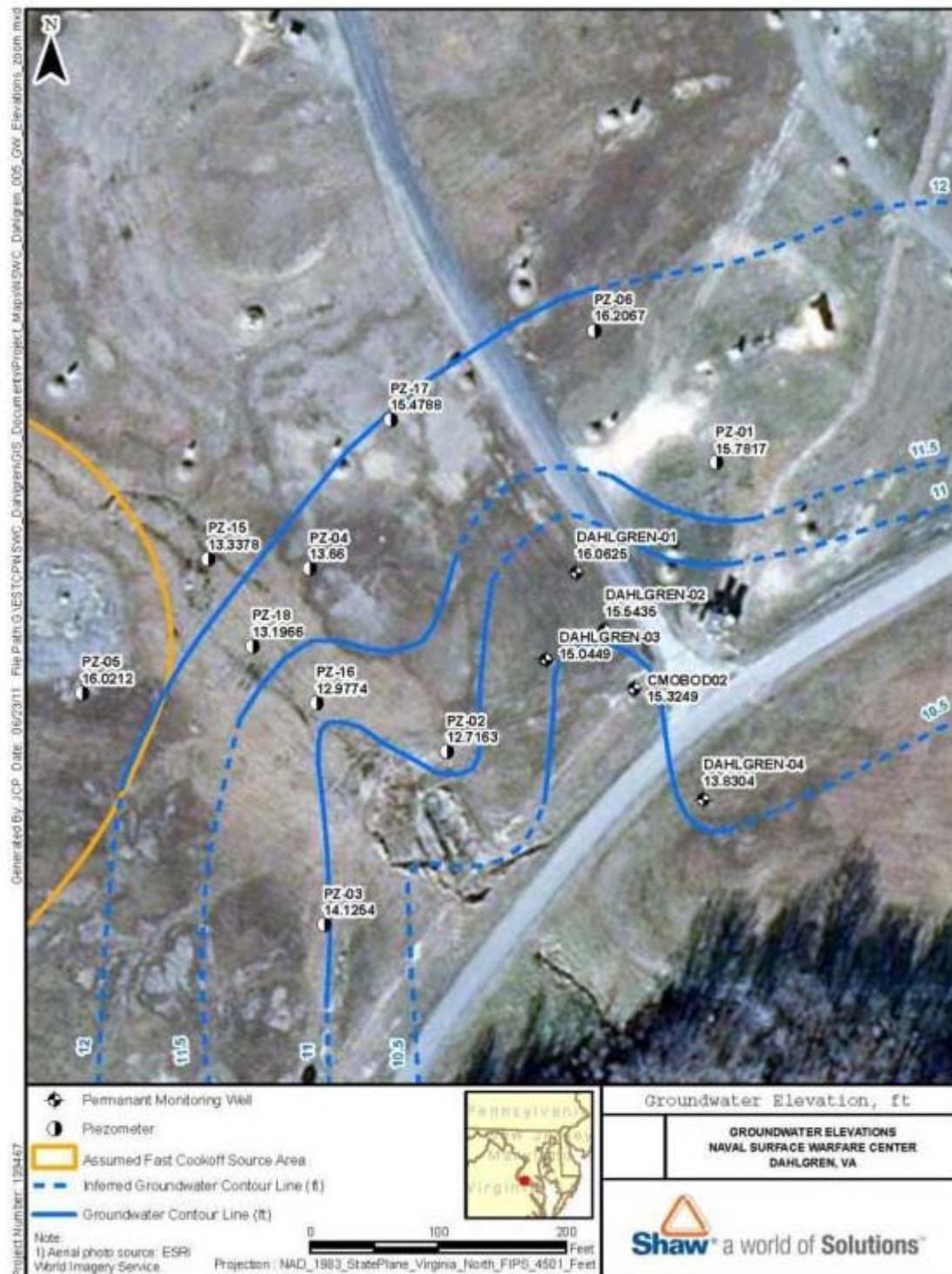
Figure 4.8. Potentiometric Surface Map of the Churchill Range in May 2011.
