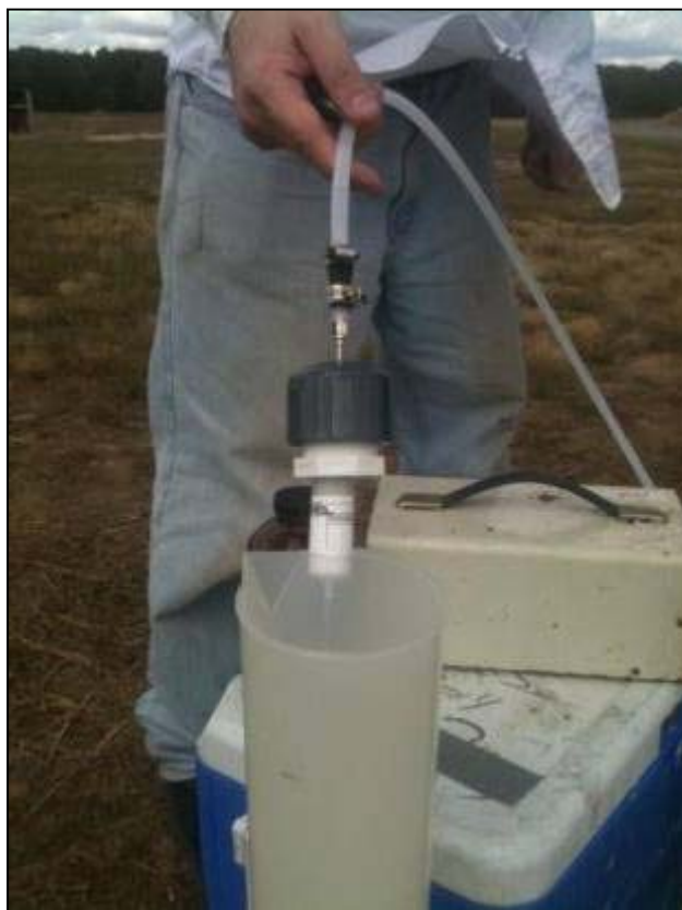
Figure 5.15. Collection of RDX for Stable Isotope Analysis on a Small SPE Column at the Dahlgren Site.
