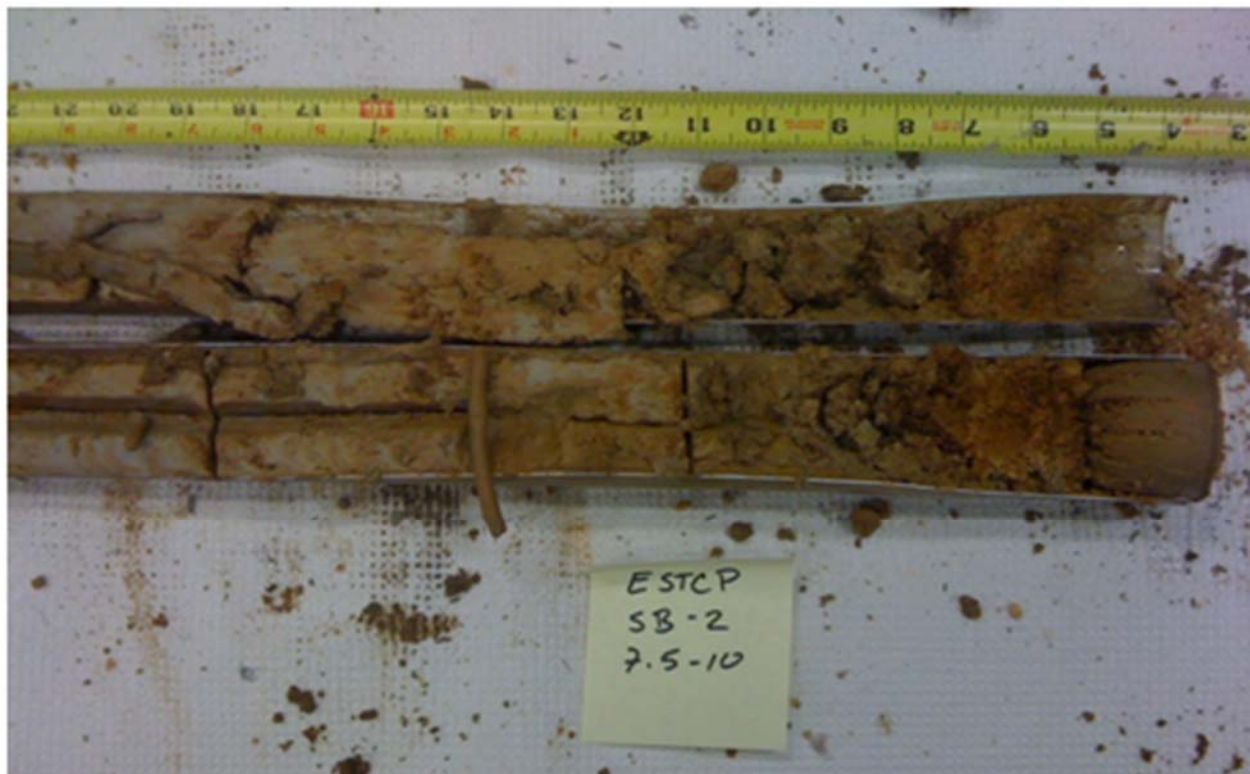
Figure 5.7. Profile of One Geoprobe Core (7.5 to 10 ft, saturated zone) from the Dahlgren Site Showing Significant Amounts of Iron Minerals (orange).
