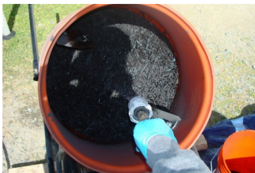
Figure 30. Inoculation of SediMite™ Pellets Prior to Deployment with VHI Device.
