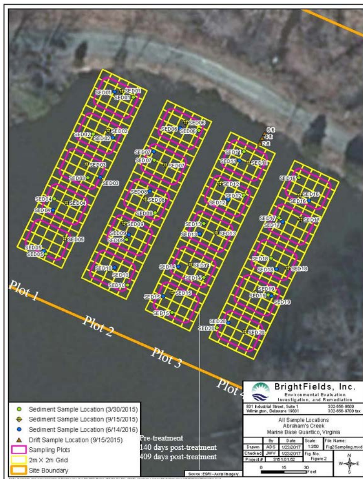
Figure 42. Sediment Sample Locations on Days 0 (pre-treatment), 140 and 409 (post-treatment).
