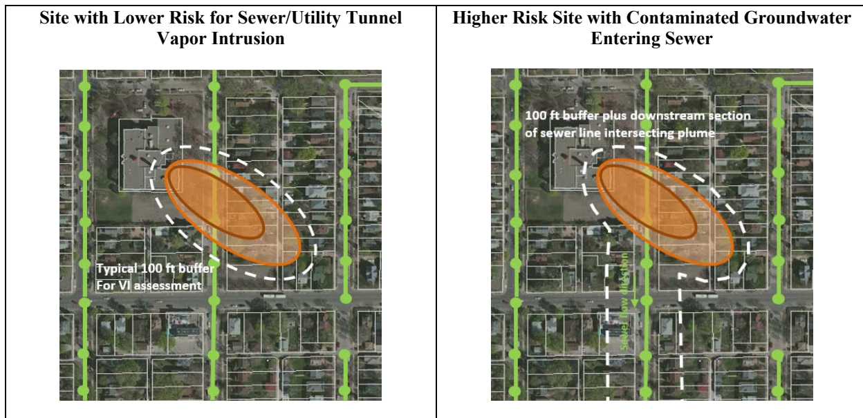
Figure 4.2 Sewer/Utility Tunnel Vapor Intrusion Risk Area
