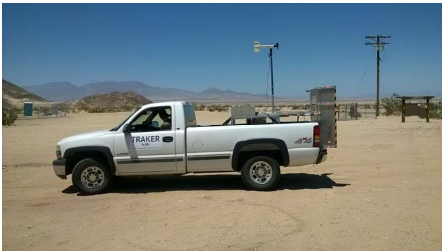
Figure 9. TRAKER™ Was Developed as a Tool to Measure Emissions of Particulate Matter (PM10 and PM2.5) Because of Vehicular Travel on Unpaved Roads.
