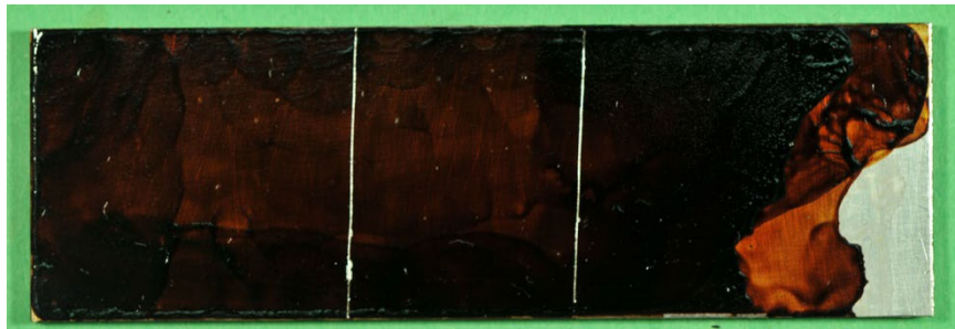
Figure 20. Panels after Wet Adhesion Tests. From top to bottom, panels A, B and C
