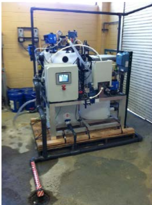
Figure 1-2. Pilot-scale electrochemical system APTIM evaluated for drinking water disinfection at Naval Air Station (NAS) Lemoore.
