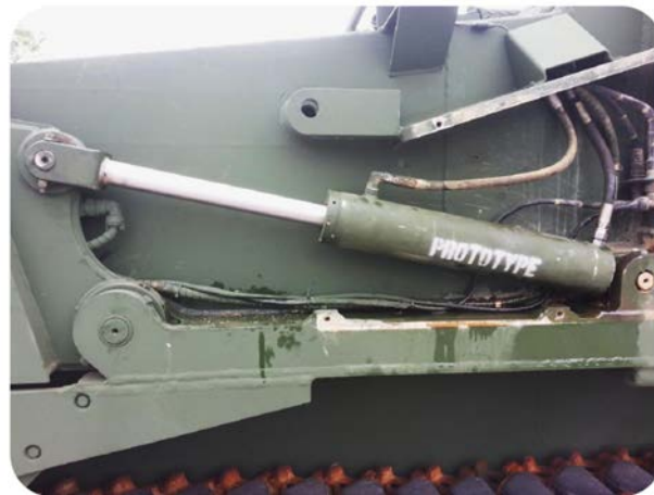
Figure 6-94. Image of installed prototype nCoP Dem/Val cylinder assembly on the M9 ACE.
