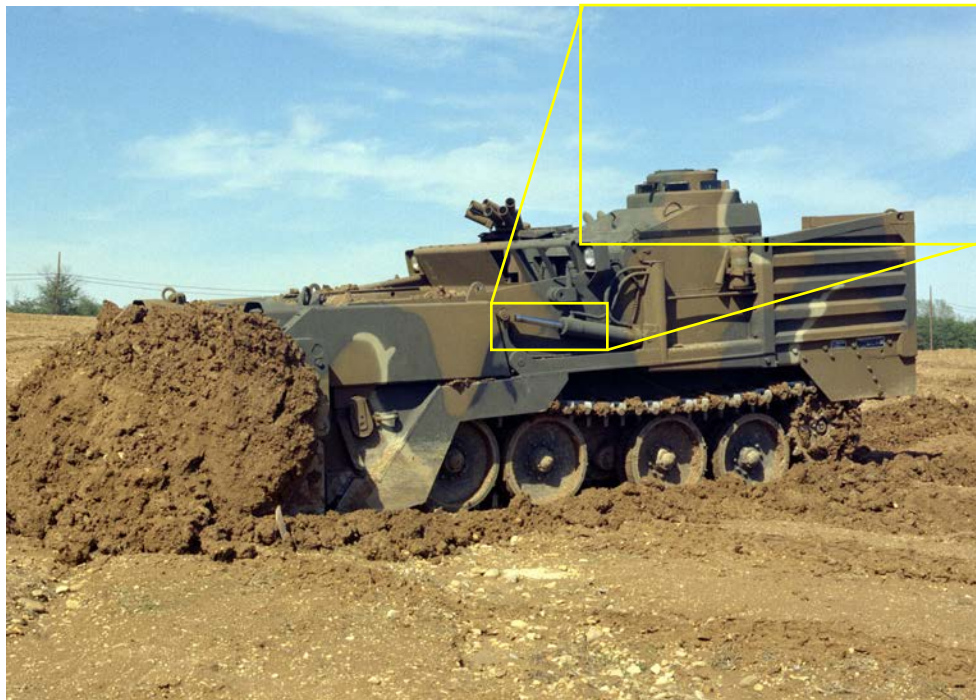
Figure 4-8. Image of M9 ACE vehicle with an inset image of the hydraulic cylinder coated with EHC plating.
