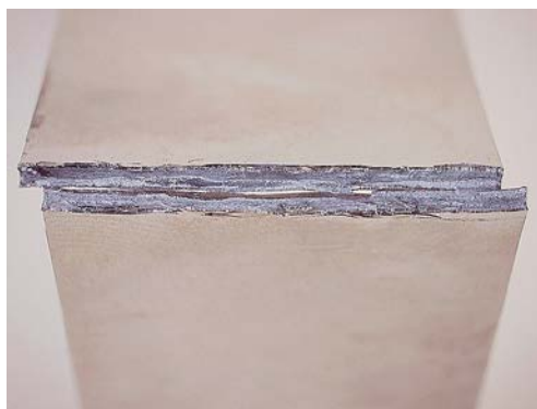
Figure 6-38. Representative image of nCoP fracture surface following bending.
