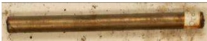
Figure 6-64. Image of nCoP sample after 720hrs in ASTM B117 showing minimal red rust.
