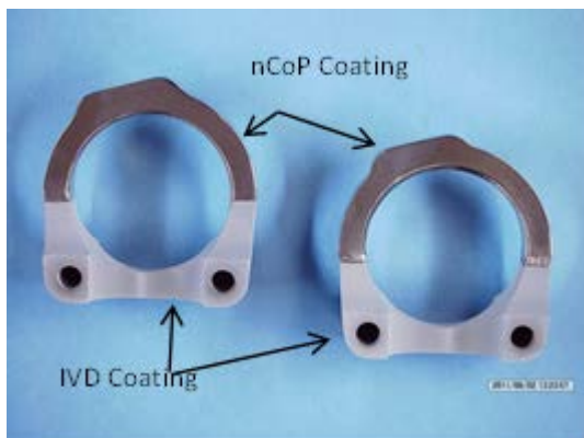
Figure 6-79. Image of nCoP and IVD Plated Tie down rings (left) and following painting Tie down rings ready for installation (right).
