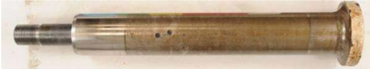
Figure 6-68. Image of nCoP Sample after hydraulic cycling with corrosion events testing.
