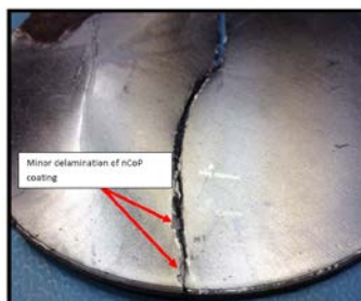
Figure 6-39. Image of Hy-tuff-2 which showed minor delamination.
