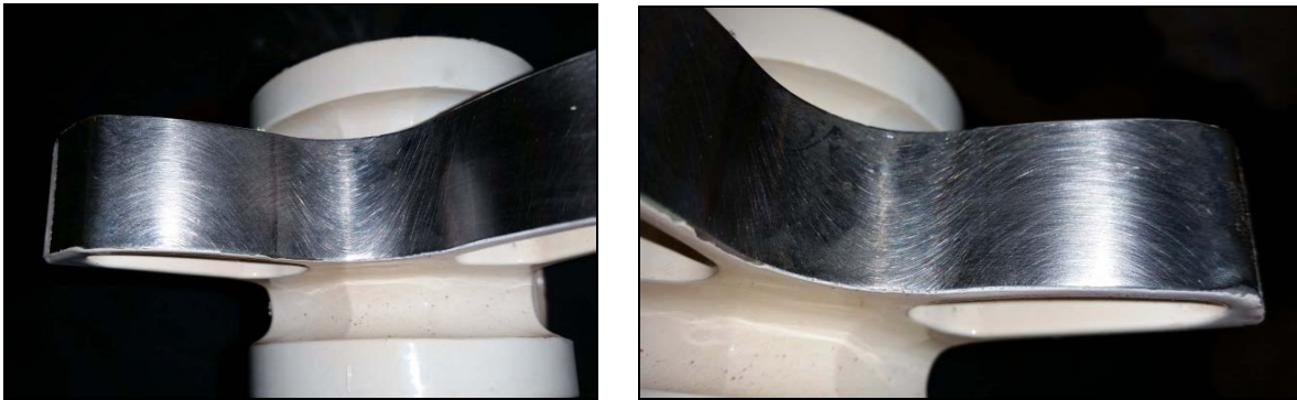
Figure 6-85. Images of cam surface of nCoP plated pivot following 97 arrestments.
