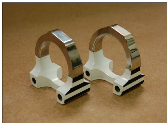
Figure 6-79. Image of nCoP and IVD Plated Tie down rings (left) and following painting Tie down rings ready for installation (right).
