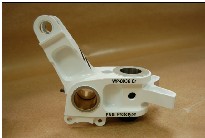
Figure 6-78. Image of EHC coated Pivot Assembly following painting front view (left) and side view (right). Stenciling of two stripes is used as identifier for field inspection.
