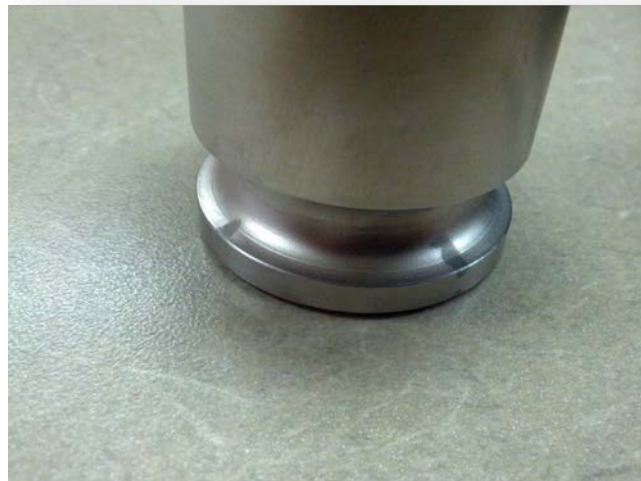
Figure 6-87. Image of Nanovate R3010 electroplated part. Grey areas are contact points which will be protected by sacrificial coating.
