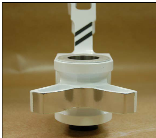
Figure 6-78. Image of EHC coated Pivot Assembly following painting front view (left) and side view (right). Stenciling of two stripes is used as identifier for field inspection.
