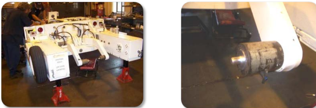
Figure 4-7. Image of lifting arm pin installed on Spotting Dolly (left) and close-up (right).
