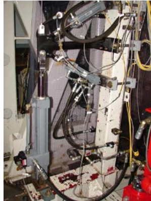
Figure 6-53. Image of the rod-seal wear testing rig at Messier-Bugatti-Dowty.
