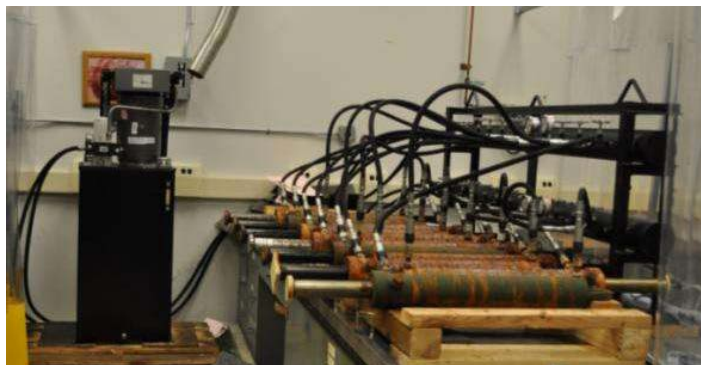
Figure 6-66. Image of hydraulic cylinder manifold with pump.
