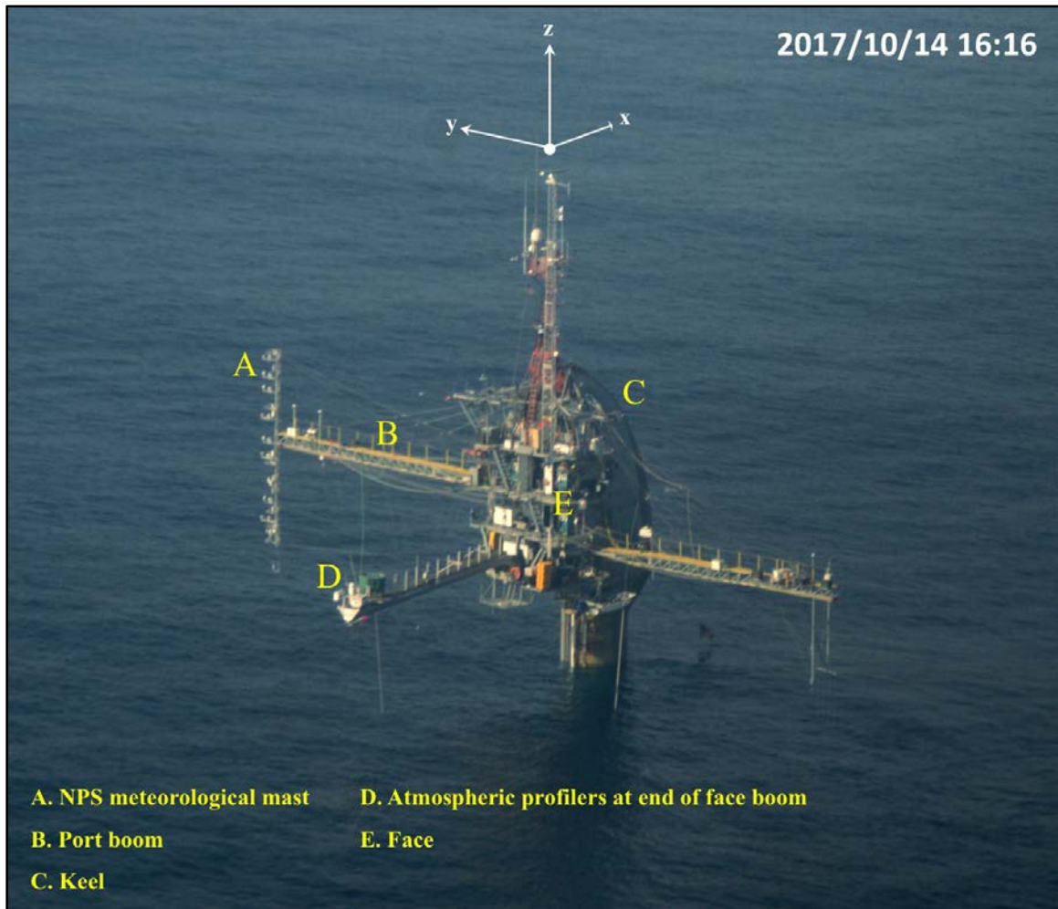
Figure 2. FLIP during the CASPER-West experiment with several features highlighted. Note that the heading of FLIP is the direction the keel points (x). The platform coordinate system is also given. Photo credit: D. Khelif, University of California at Irvine.
