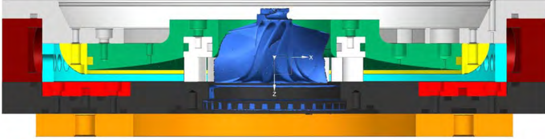
Figure 24. RRDE with turbine integrated in place of nozzle. Image courtesy of R. Huff, AFRL/RQTC.
