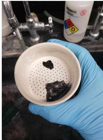
Figure 36. Carbon fibers and CNT clump after nitric acid digestion of the cyanate ester resin.
