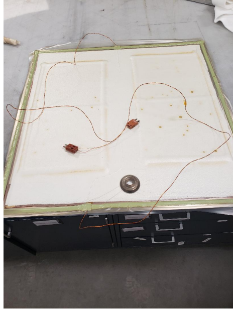
Figure 32. Four panels packaged for autoclave cure.
