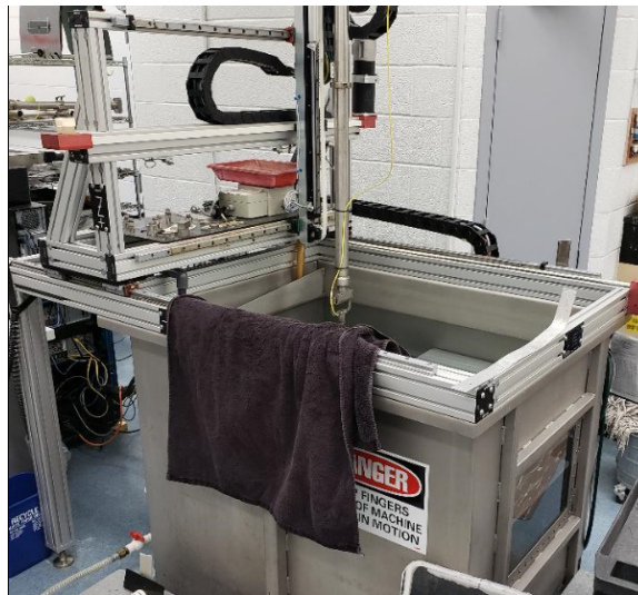
Figure 31. Wesdyne ultrasonic scan equipment used to map the density of the composite panels. This was used for ensuring good consolidation of the panels from autoclave curing as well as for determining delamination area in the panels after ballistic impact.
