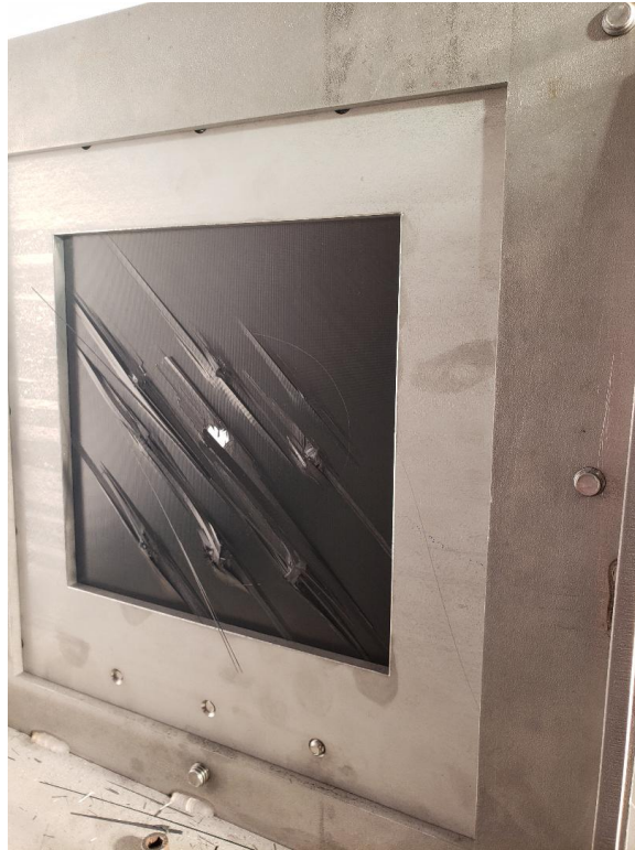
Figure 69. Back-face delaminations from V50 testing of panel 1.2
