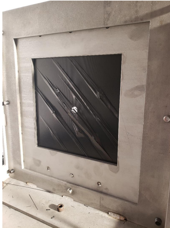
Figure 68. Back-face delaminations from V50 testing of panel 1.2
