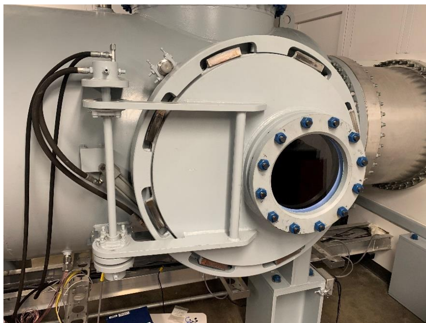
Figure 9. Autoclave door with optical access
