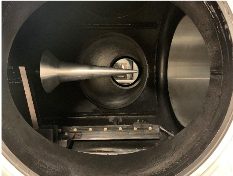
Figure 17. Model positioned in test section (43° base and 10.2mm tip installed)
