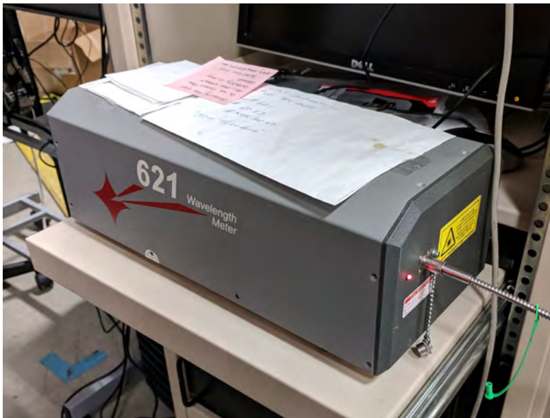
Figure 37. Bristol Model 621 wavemeter, fiber-coupled to the LAS system.
