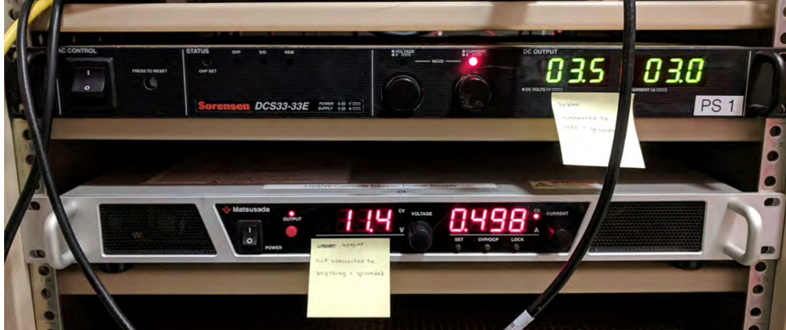
Figure 19. Matsusada REK650-2.5 power supply, used to power the cathode keeper, and Sorensen DCS33-33E power supply, used to power the cathode heater.
