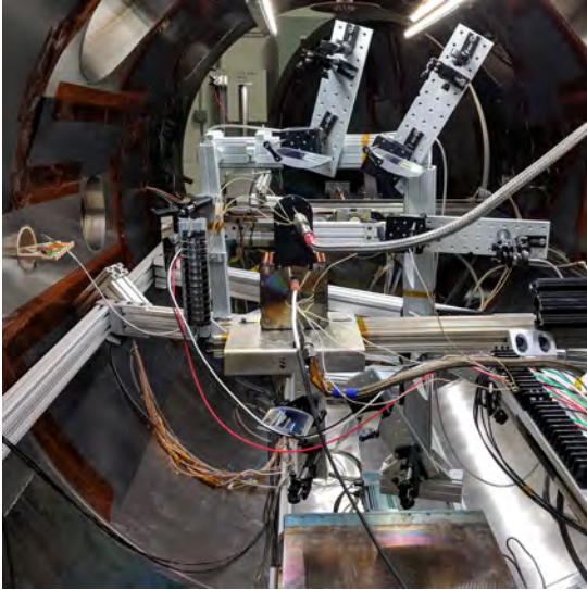
Figure 35. Mounted Busek BHT-600 Hall thruster with BHC-1500 hollow cathode, and LAS system optic assembly, viewed from the rear.
