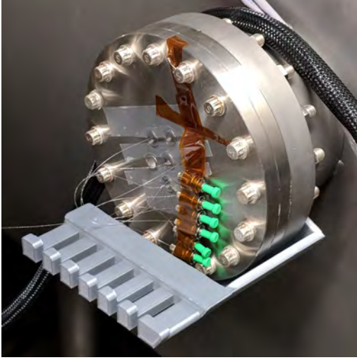
Figure 26. Custom fiber pass-through, exterior, with strain relief.
