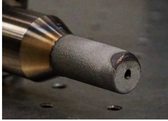
Figure 7. Hollow cathode erosion, with visible degradation of the orifice and cathode keeper.
