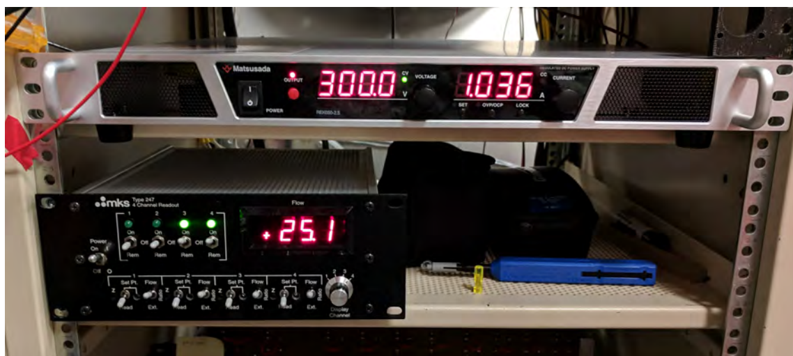
Figure 18. Matsusada REK650-2.5 power supply, used to power the anode. Also pictured, MKS Type 247 mass flow readout.
