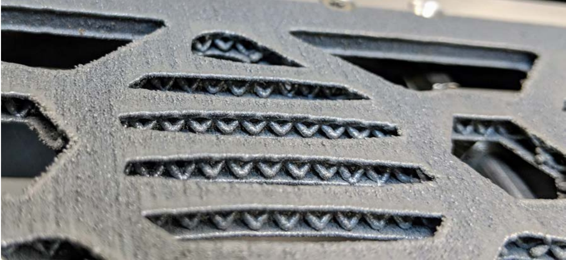
Figure 4.1. AlSi10Mg Lattice Based CubeSat Chassis [11]
