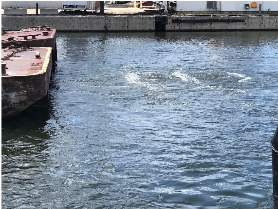
Figure 14. Visible turbulence from CSSC water jet, fish entrainment control measure testing, August 23, 2017.
