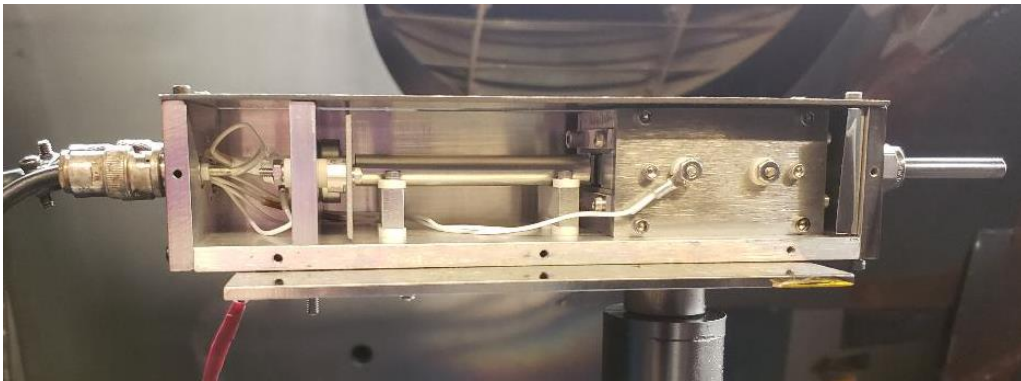
Figure 23. E \times B Probe with Exterior Shielding Removed
