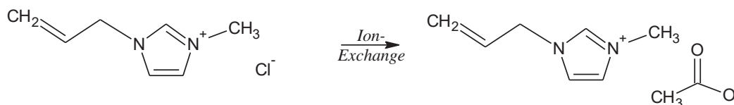
Figure 6. Ion exchange process for generation of AMIAc (right) from AMICl (left).
