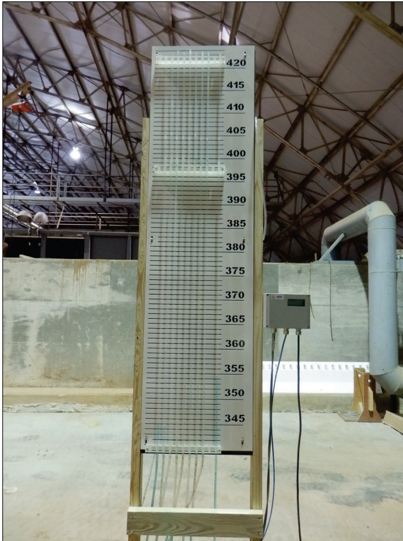
Figure 14. Piezometer display board.
