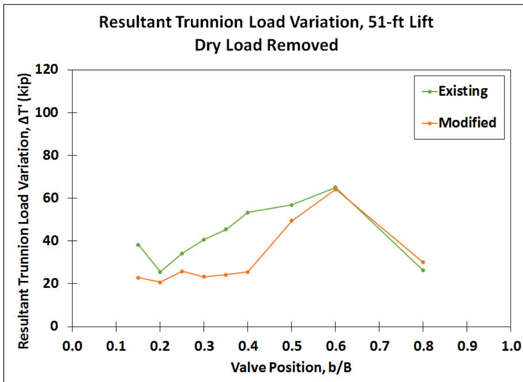
Figure 88. Resultant trunnion load variation between valves – 51 ft lift.
