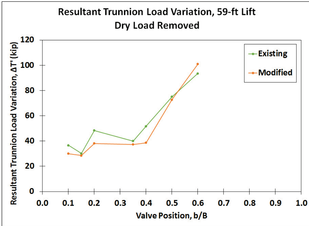
Figure 89. Resultant trunnion load variation between valves – 59 ft lift.
