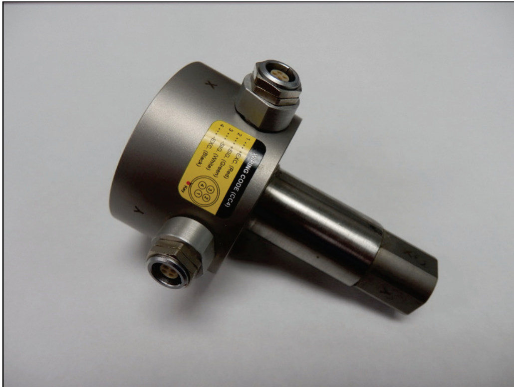
Figure 18. Trunnion load measurement instrument.
