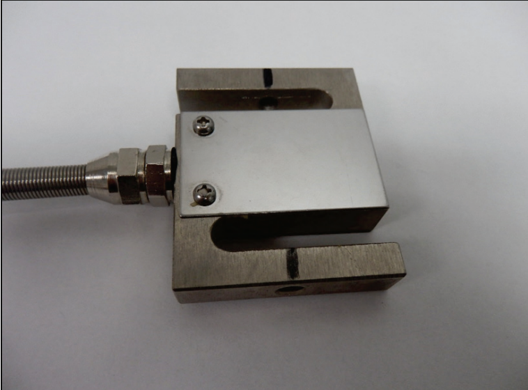
Figure 16. Hoist load (force in long strut) measurement instrument.
