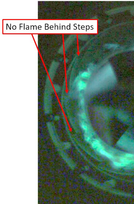
Figure 98: Circumferential cavity combustion 0.273 seconds prior to flameout
