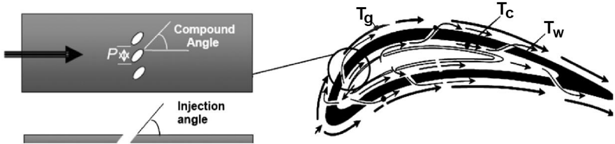
Figure 19: Turbine blade cross section depicting film-cooling airflow [29]
