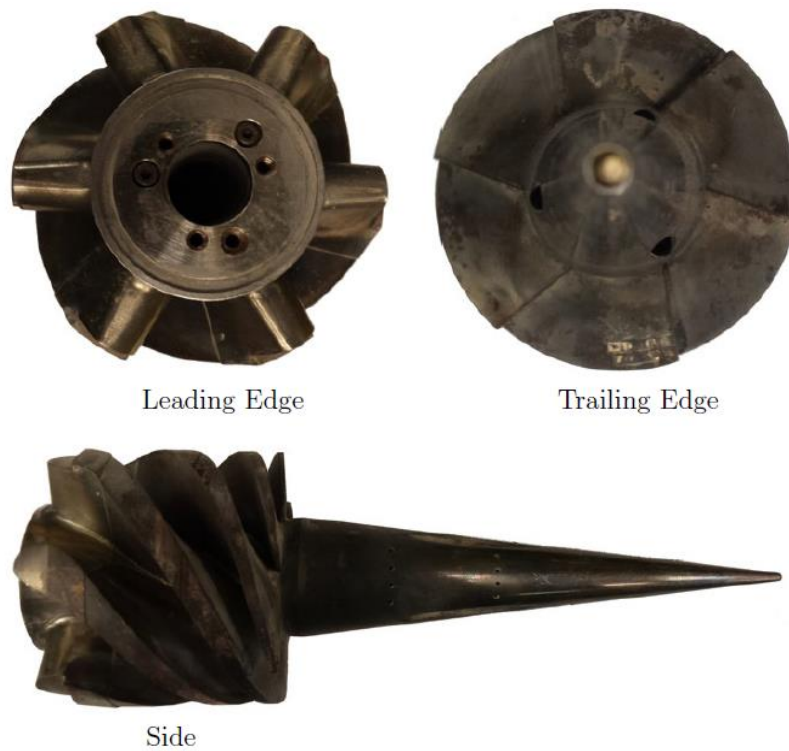
Figure 44: Solid HGV geometry [5]
