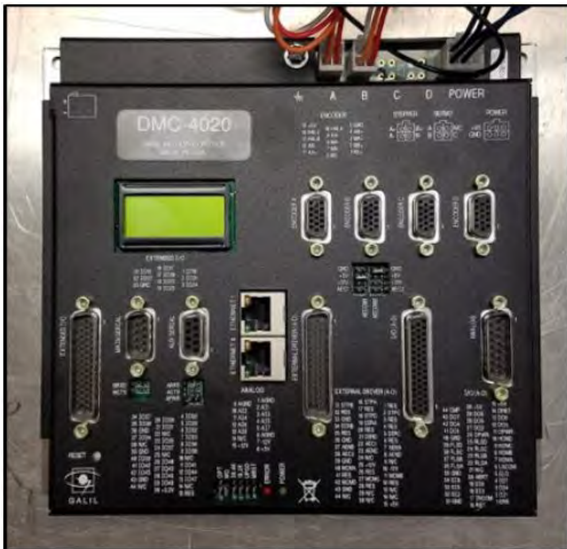
Figure 26: Galil DMC-4020 dual-axis motion controller [8]
