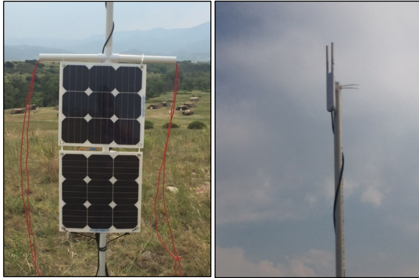
Figure 24. Solar Panel Mast and Top View of Field Node
