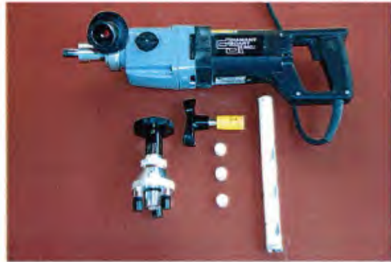
Adhesion tester, air-cooled core drill, core bit, and pull-off coupons.
