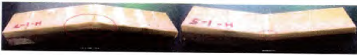
Figure 43. Specimens post-testing. Back side of the specimens are shown to help distinguish between the composite and aluminum layers. Damage is highlighted with red circles and lines to illustrate where the damage occurs. (Left) Composite in tension, specimen-format A. (Right) Composite in compression, specimen-format B.
