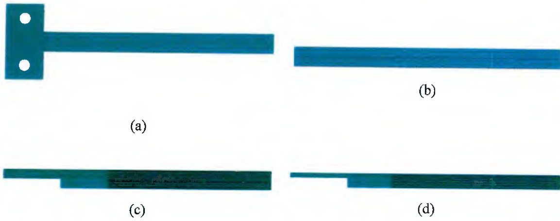
Figure 37. FE models for the DCB (a), ENF (b) and SLB (c, d) tests
