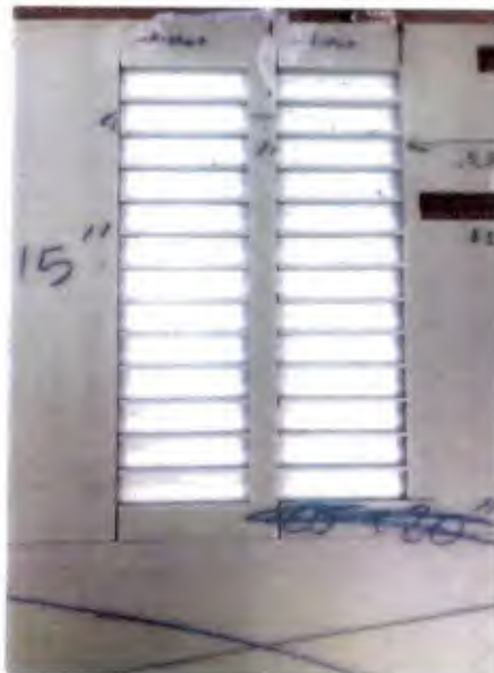
Figure 41. Metal/composite hybrid plate with specimens cut out. Delamination is shown near the initial lead-in (top). The first several specimens were invalid.
