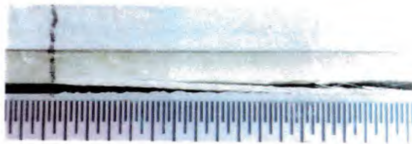
Figure 62. Interface disbond initiating at multiple locations.
