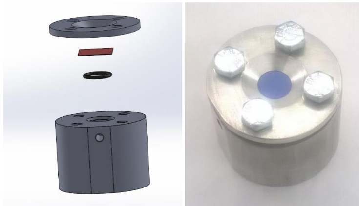
Figure 2 Sample holder for testing rubber membrane using a dynamic micro-fringe projection system.
