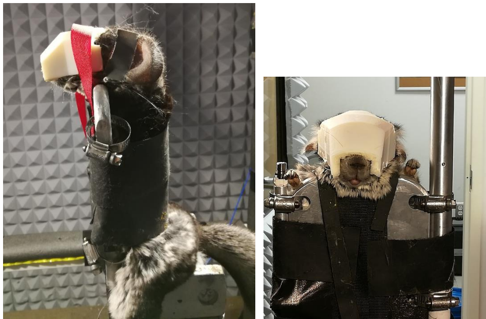
Fig. 23. View of a chinchilla with the prototype helmet for blast test inside the test chamber. Left: side view; Right: front view.
